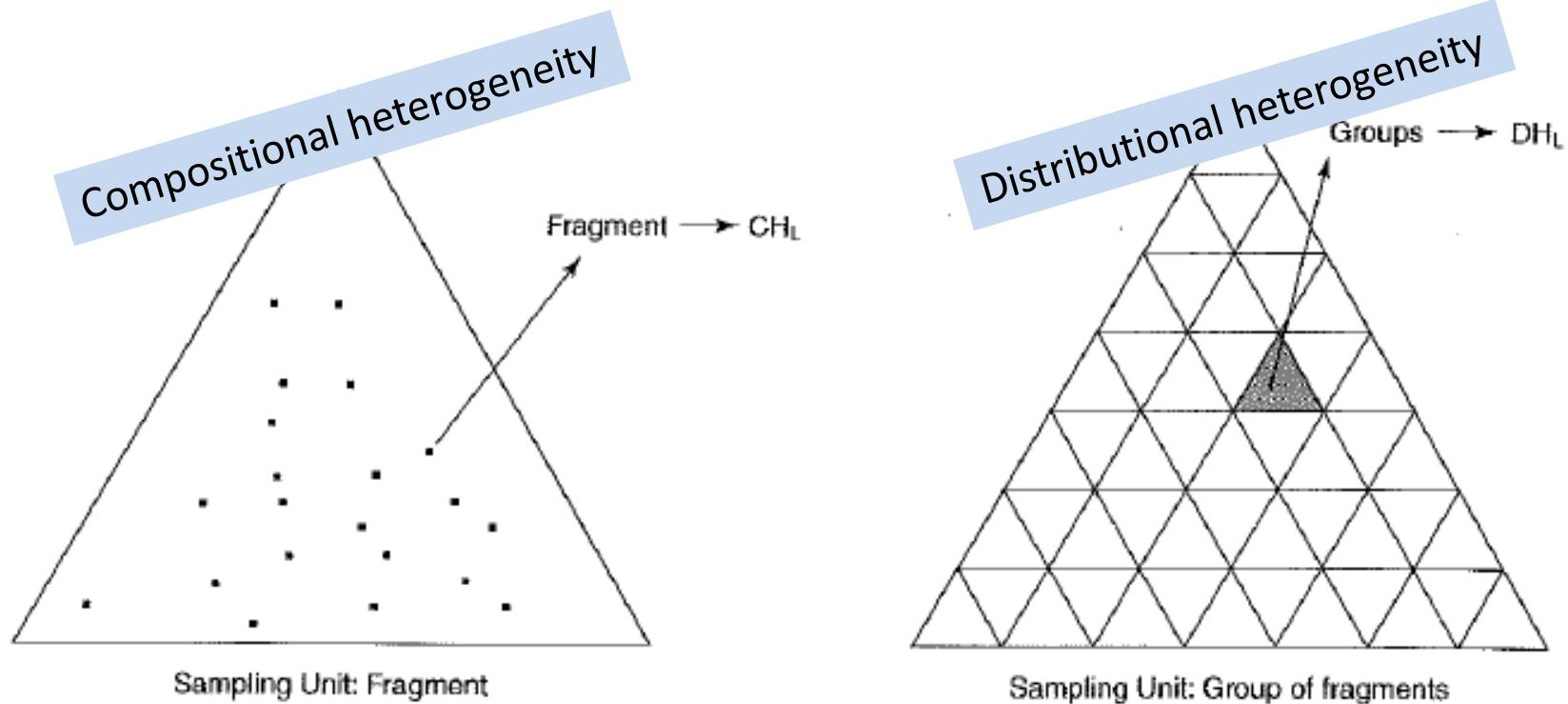
**Figure 3.1** Principle illustration of scale-related concepts of constitutional and distributional heterogeneity. The constitutional heterogeneity, CH<sub>L</sub>, expresses all between-fragment compositional differences in the entire lot, while the distributional heterogeneity, DH<sub>L</sub>, reflects all between-increment (between-group) compositional differences, which can be seen as covering the entire spatial geometry of the lot.
